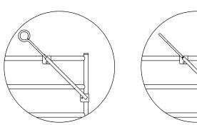
With the Latch Rod positioned as shown, it will hold itself in place and stay clear when the gate is swung open.
