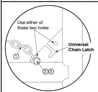
**NOTE:** For the safety of your horse, make sure the nut is located to the outside of the enclosure.
