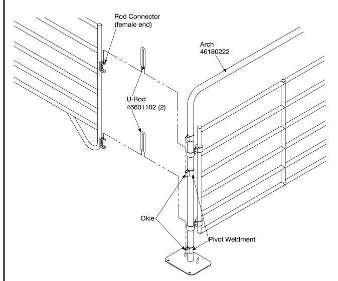
Using the two U-Rods provided, attach the Corral Panel with the Rod Connector - female end (Do **NOT** use side with the pin and chain weldment) to the Okies on the Pivot Weldment on the Arch Gate as shown.
