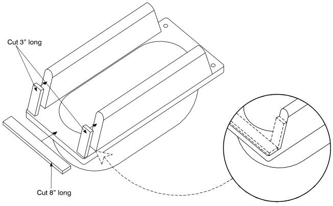
Peel off backing of self-adhering weatherstrips and apply to both sides of Inspection Cover.
