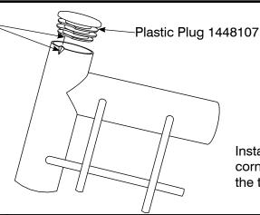
Install Plastic Plugs on all **top** corners of the kennel including the tops of the door(s).
