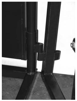
4. Next, position the A.I. Cage (62178422) until the top hookups align and then insert the pin as shown.
