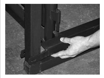
6. Next, slide the adaptor upwards and against the Crowd Alley Frame until the bottom of the A.I. Cage pin is connected into the hookup. Place one (1) hex bolt (3188031) with one (1) washer (3948003) in each side through A.I. Cage Adaptor slots and securely fasten using one (1) hex nut (2688008).
