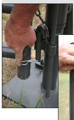
Connect alley exit panel to center assembly. Be sure and insert R-pins in the bottom of the attachment pins.
