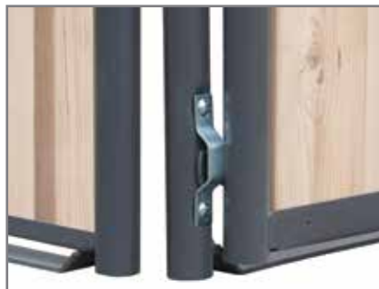
Reversible latches allow stall to be easily configured as right or left entrance.
